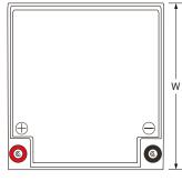
L: 6.55 (166.5) W: 6.88 (175) H: 4.64 (118) HT: 4.92 (125) Tolerances are +/- 0.04 in. (+/- 1mm) and +/- 0.08 in. (+/- 2mm) for height dimensions. All data subject to change without notice.
